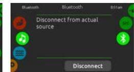
If a device with Bluetooth technology is connected to the in.stream 2, you can disconnect it by pressing the Disconnect key at the bottom of the screen.
