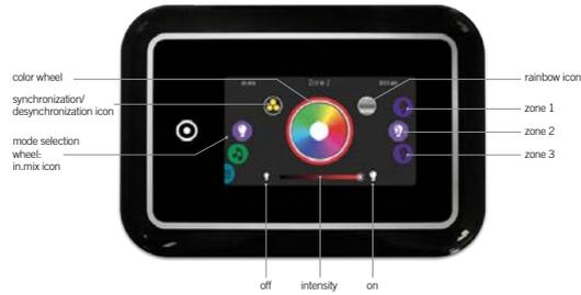
To select the color mode, slide the left wheel up or down until the in.mix icon menu is highlighted in the middle.
